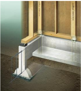
Foundation direct joints
